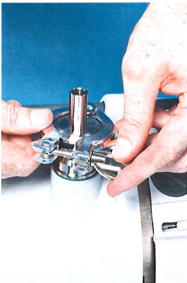
(C) • Swing clamp around inlet port adaptor
