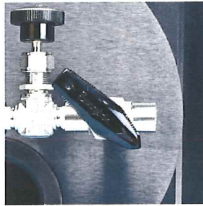
(B) • 3-way valve partially open to inert gas
