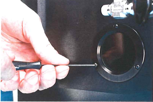
(A) • Remove the three (3) screws
