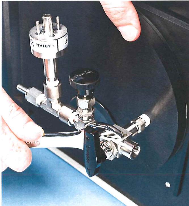
Figure 10 • Connecting the Vacuum Gauge Assembly and Needle Valve/3-Way Valve Assembly to the Plasma Cleaner Door
