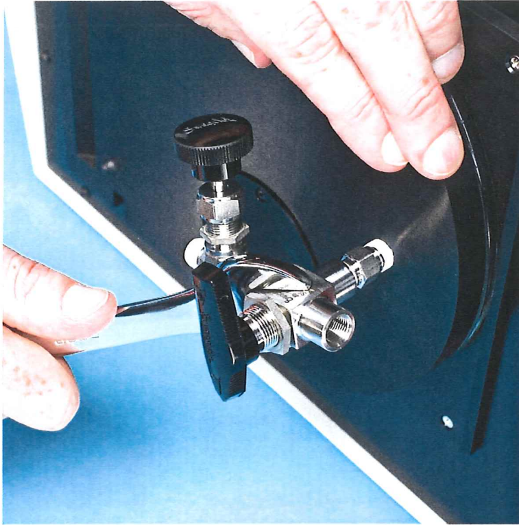
Figure 5 • Connecting the Needle Valve/3-Way Valve to the Plasma Cleaner Door
