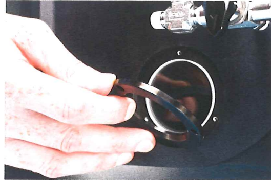
(B) • Remove the retaining ring
