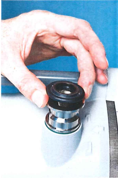
(A) • Centering ring on the inlet port
