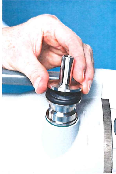
(B) • Adaptor on the inlet port
