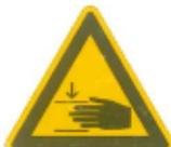
Please be aware of injury risk in case of inappropriate handling, especially the insertion of fingers/hand into the crimping jaws or between the crimping handles during the crimping process. Compress at the end of the handles to optimise the applied crimping force. Please use eye protection and proper attire all the time!
